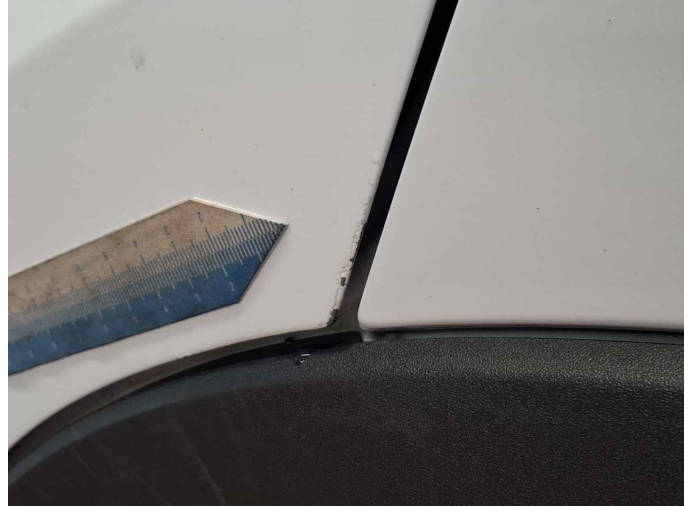
Damage 6: Door - rear left side: Door edge - Scratch(es) - Smart repair
