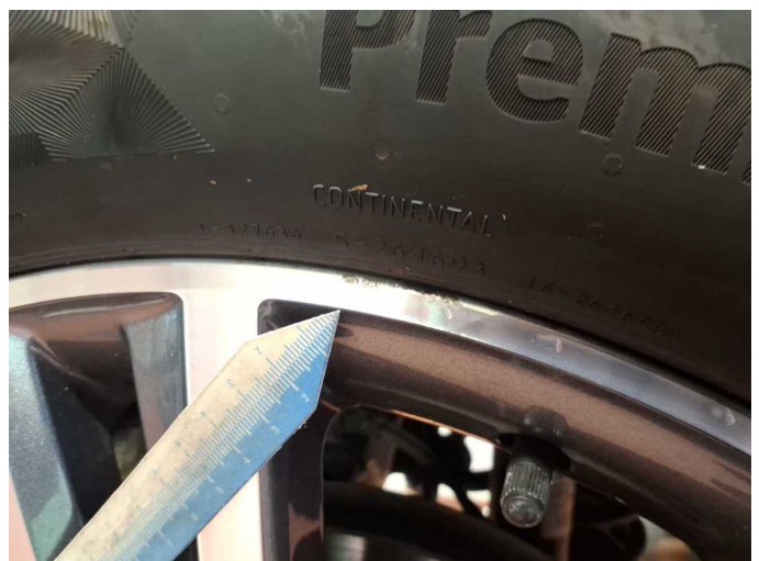
Damage 7: Wheel / tyres: Alloy rim - rear left side - Scratch(es) - Loss in value
