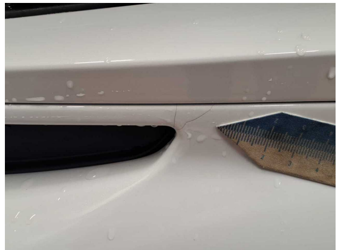
Damage 4: Front bumper: Spoiler - Scratch(es) - Smart repair
