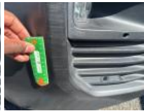
Bumper F, Scratch(es), Repair and paint (complete)
