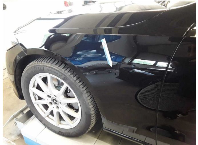
Damage 6: Mudguard - left side: Mudguard - left side - Dent / paintcoat damage - Repair and paint
