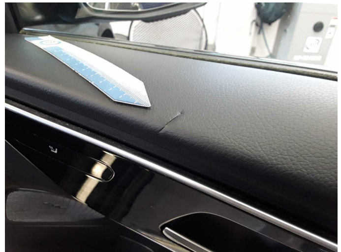
Damage 4: Trim / covers: Door trim - front right side - Damaged - Smart repair
