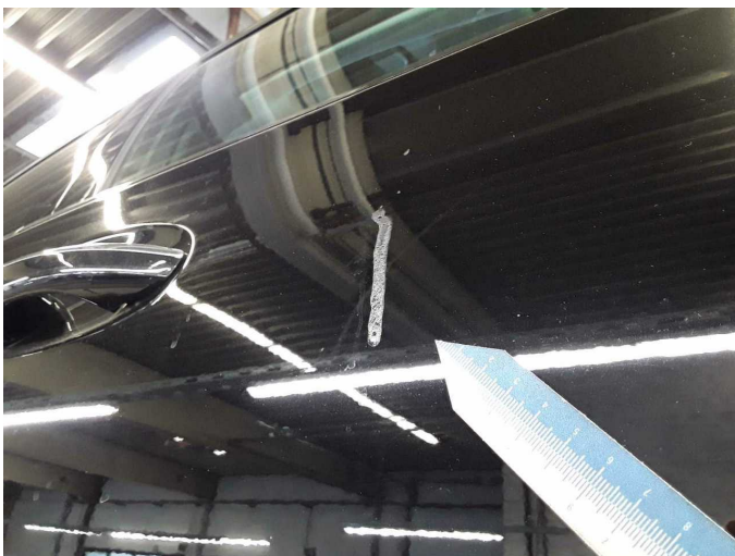
Damage 2: Door - front right side: Door (Harztropfen) - Paint defect - Smart repair
