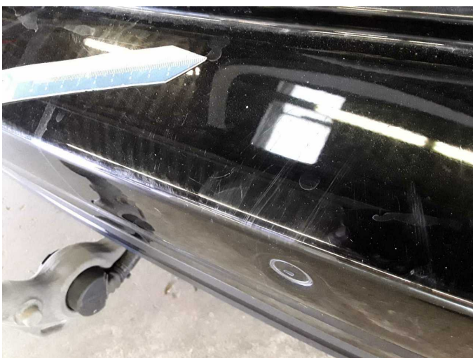
Damage 9: Rear bumper: Rear bumper - Scratch(es) - Paint
