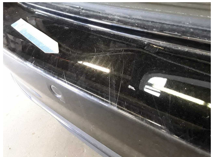
Damage 9: Rear bumper: Rear bumper - Scratch(es) - Paint
