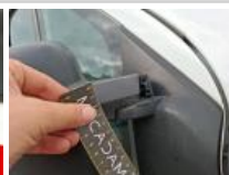
Side panel moulding R, Broken, Replace
