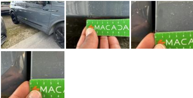
Door trim RR, Scratch(es), Paint
