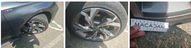
Tyre FR, Tear, Replace
