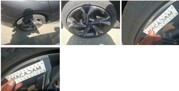
Tyre RR, Tear, Replace
