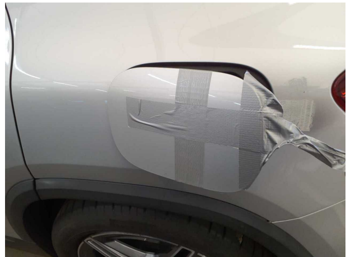
Damage 3: Fuel system: Tank flap - Broken / torn - Replace
