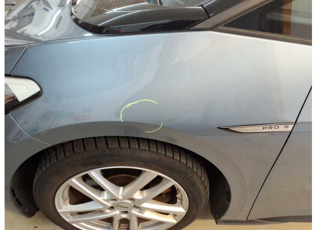
Damage #6: Mudguard - left side: Mudguard - left side - dent(...) - Smooth repair work
