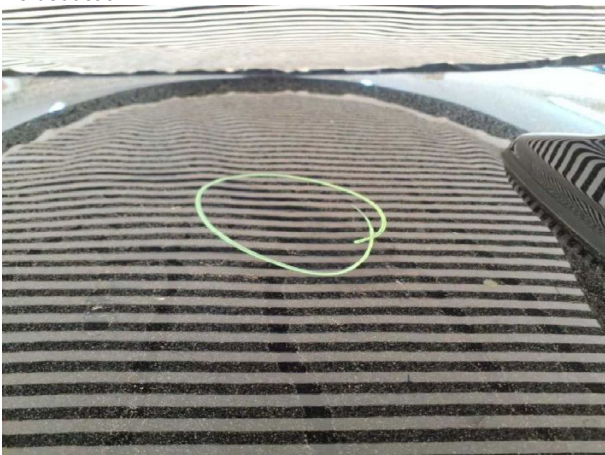
Damage #4: Roof: Roof - dent(s) - Smooth repair work
