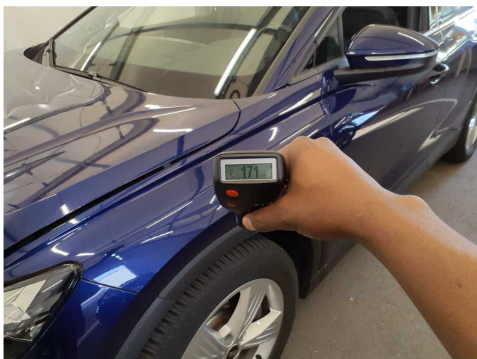
Repainting 1: Mudguard - left side
