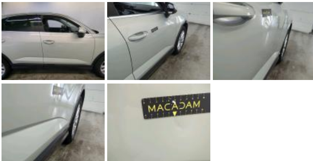
Wing FR, Dent(s) and scratch(es), Repair and paint (complete)
