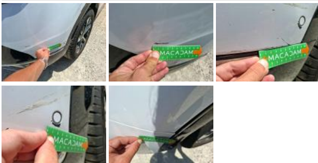
Bumper spoiler Rear, Broken, Replace
