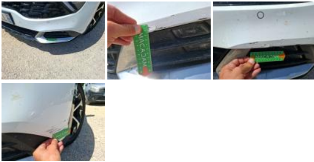
Bumper moulding FL, Broken, Replace
