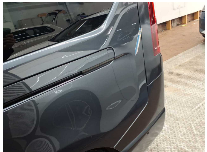
Damage 4: Side panel - rear left side: Side panel - dent(s) - Repair and paint
