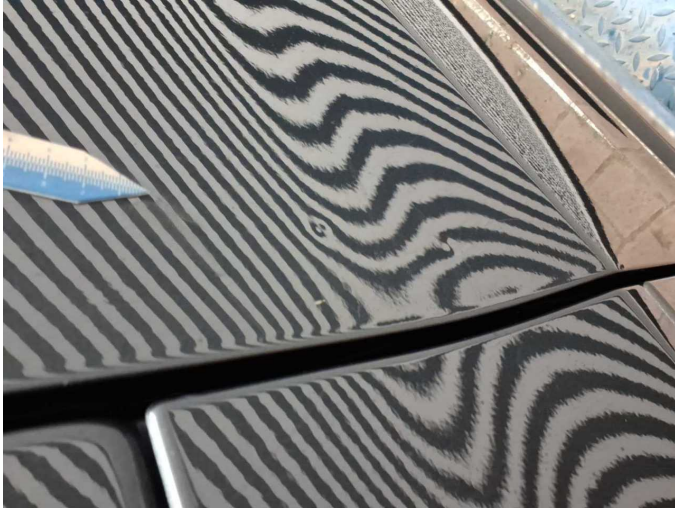
Damage 6: Door - rear left side: Door (Und kratzer) - dent(s) - Repair and paint
