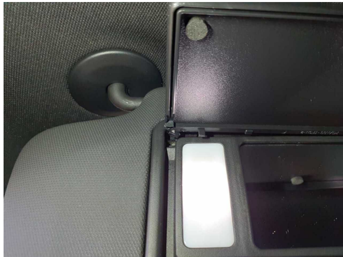
Damage 5: Interior: Sun visor - left side - Broken / torn - Replace
