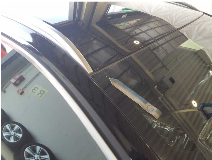
Damage 8: Vehicle glazing: Windscreen - Stone chips - Replace
