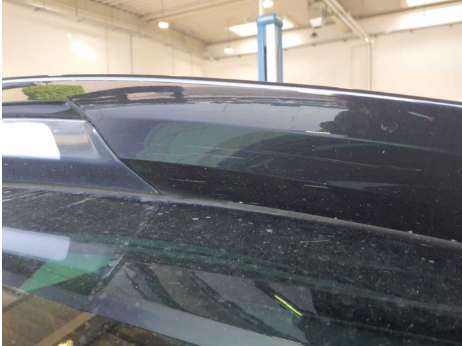
Damage 1: Boot lid / rear door: Rear spoiler - Scratch(es) - Smart repair
