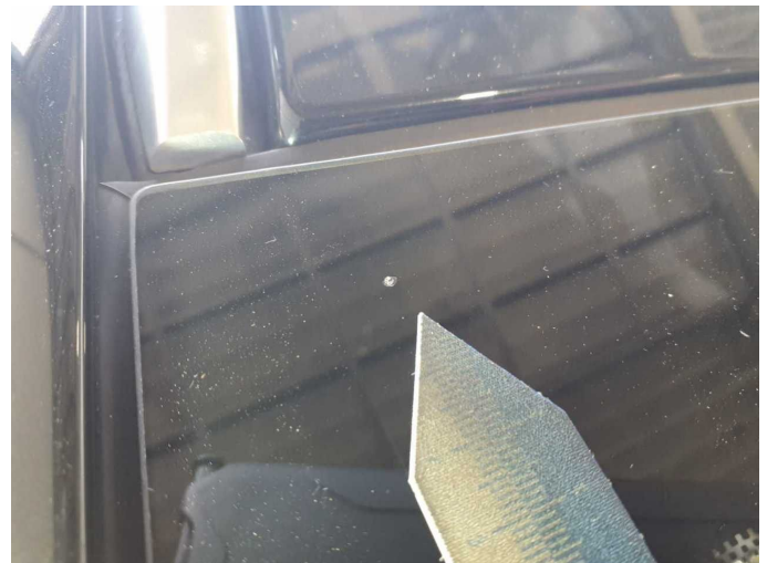
Damage 8: Vehicle glazing: Windscreen - Stone chips - Replace
