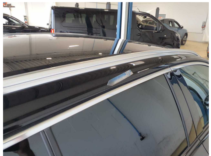
Damage 4: Roof: Roof rail - right side - Scratch(es) - Smart repair
