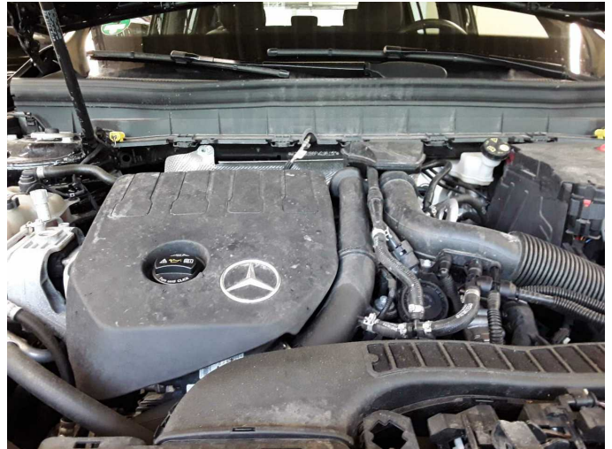
Damage 1: Engine: Engine cover - Damage caused by marten / rodent - Replace
