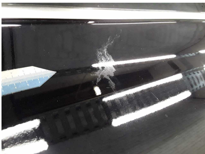
Damage 3: Side panel - rear right side: Side panel (Vogelkot eingebrannt) - Paint defect - Paint
