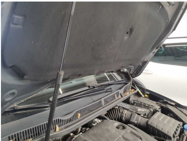
Damage #2: Bonnet: Insulation lining - Loose - Un- / install
