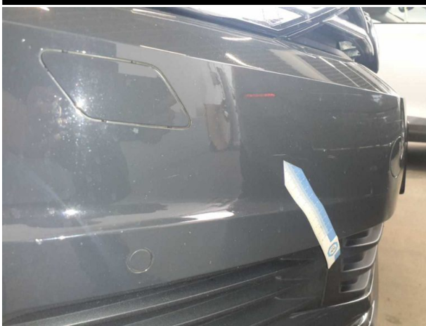
Damage #5: Front bumper: Front bumper - Scratch(es) - Paint
