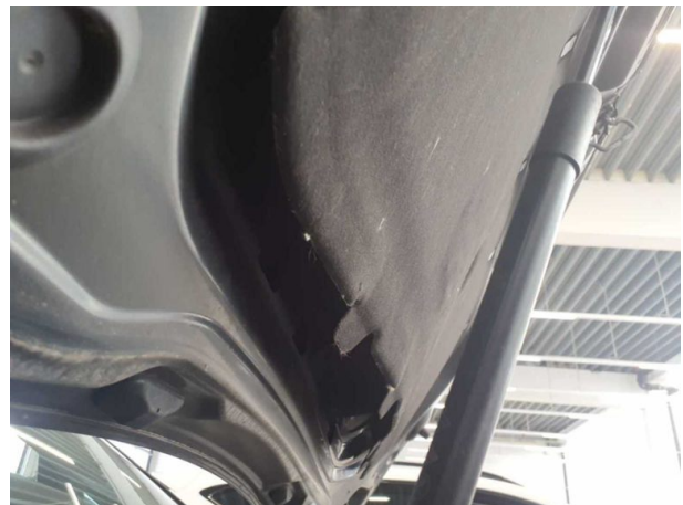
Damage #2: Bonnet: Insulation lining - Loose - Un- / install
