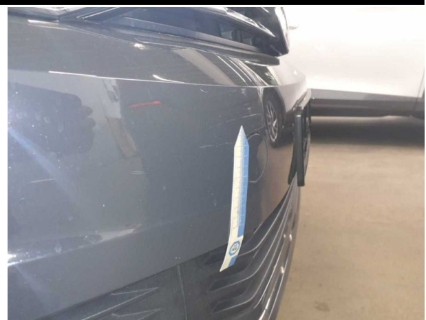
Damage #5: Front bumper: Front bumper - Scratch(es) - Paint
