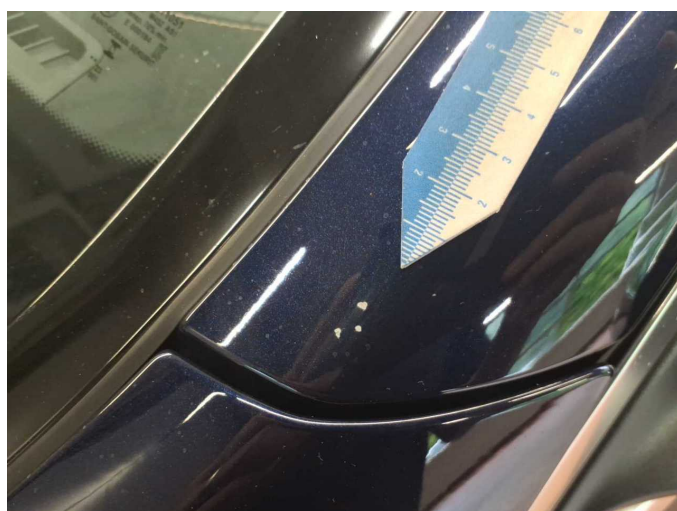
Damage 4: Roof: Roof rail - left side - Stone chips - Smart repair
