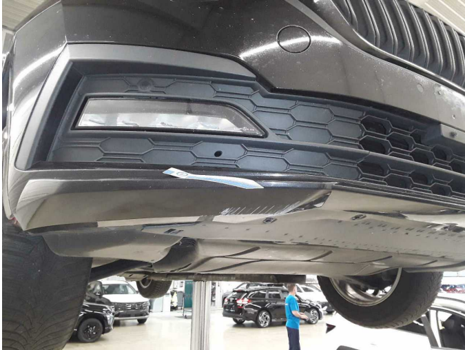
Damage 6: Front bumper: Spoiler - Scratch(es) - Smart repair
