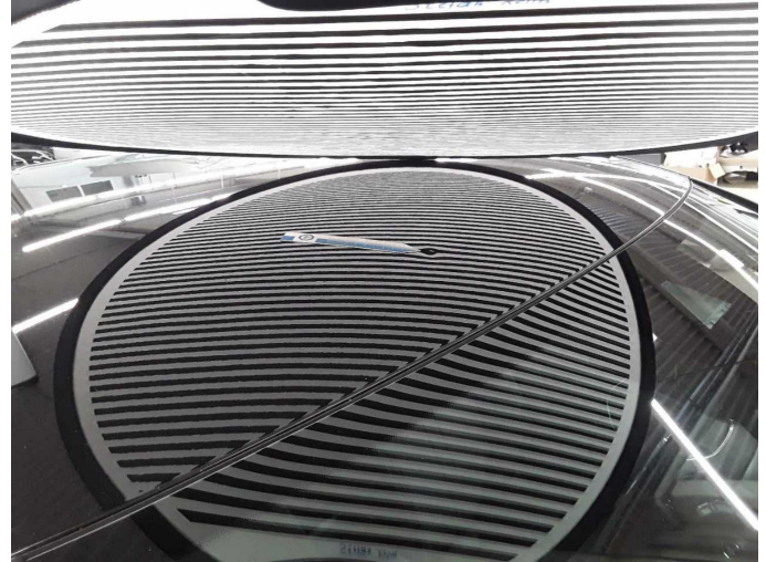
Damage 2: Roof: Roof - dent(s) - Smart repair
