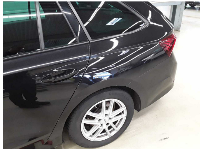
Damage 9: Side panel - rear left side: Side panel - Scratched - Repair and paint
