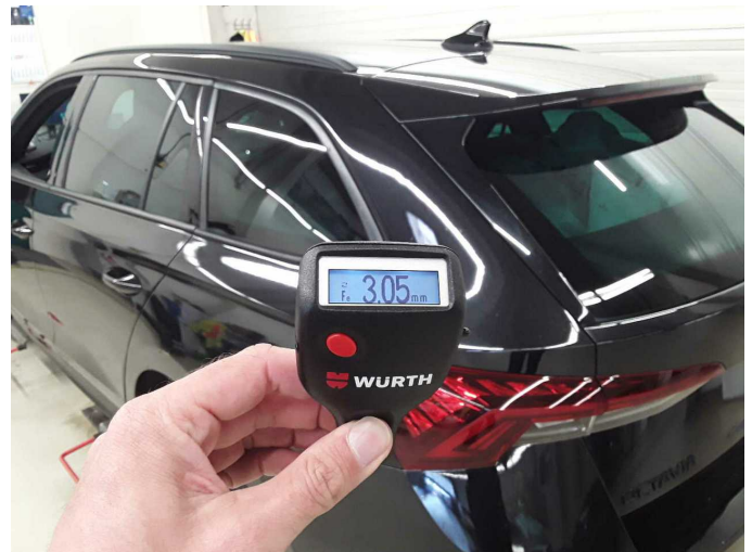
Side panel - rear left side: 3,050 \mu\text{m}
