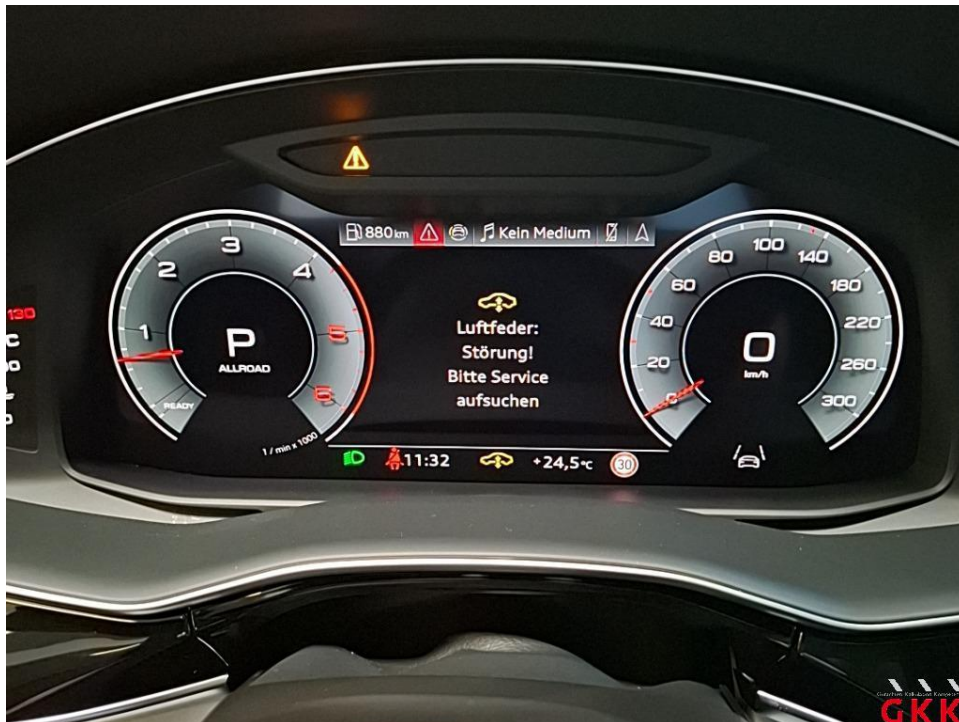
Picture 20 chassis, level regulation, functioning, inspect
