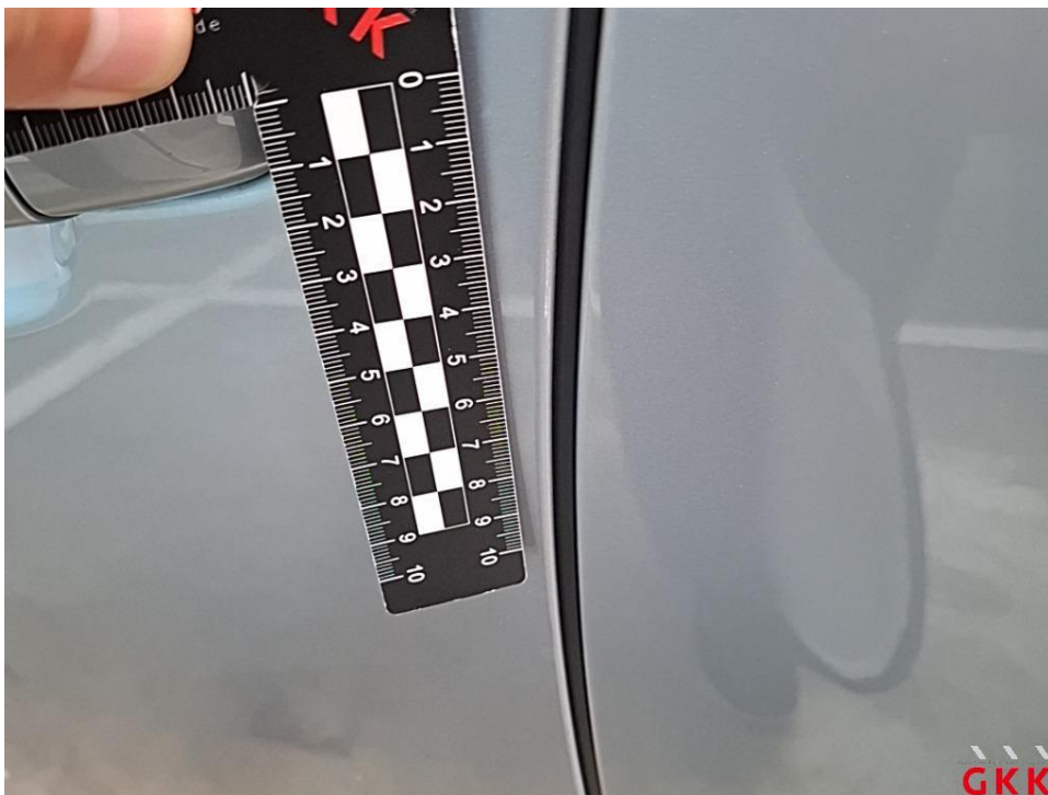
Picture 22 door front left, edge, scratched, disassemble, grind, polish
