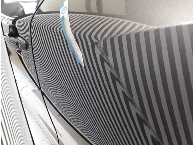
Damage 5: Door - rear left side: Door - Dent / paintcoat damage - Paint
