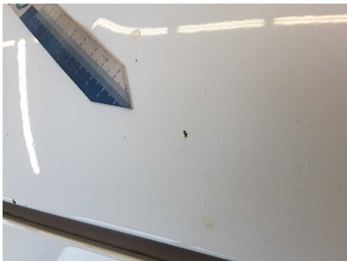
Damage 5: Bonnet: Bonnet - Corrosion - Repair and paint
