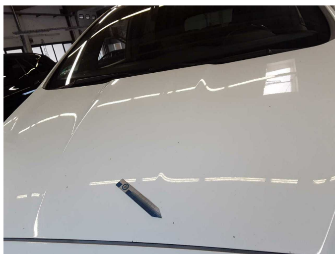
Damage 5: Bonnet: Bonnet - Corrosion - Repair and paint
