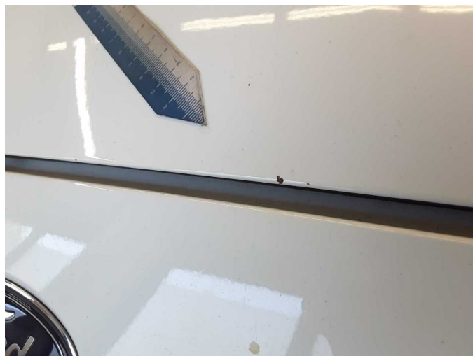
Damage 5: Bonnet: Bonnet - Corrosion - Repair and paint
