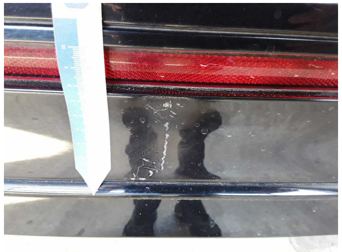
Damage 2: Rear bumper: Rear bumper - Scratch(es) - Paint
