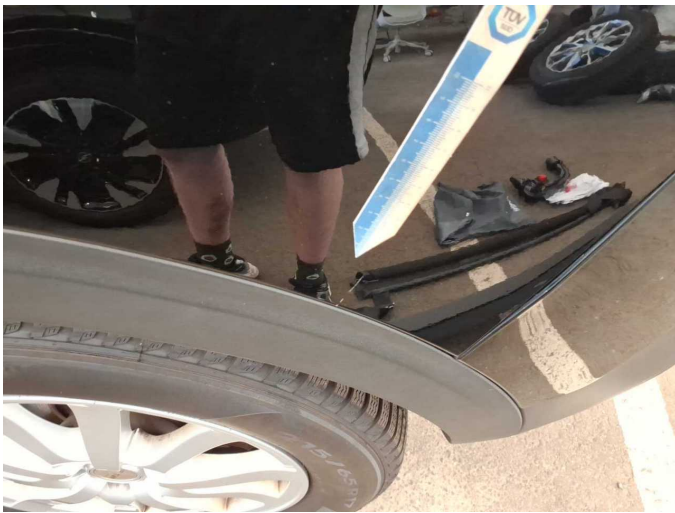
Damage 4: Side panel - rear left side: Side panel - Scratch(es) - Paint
