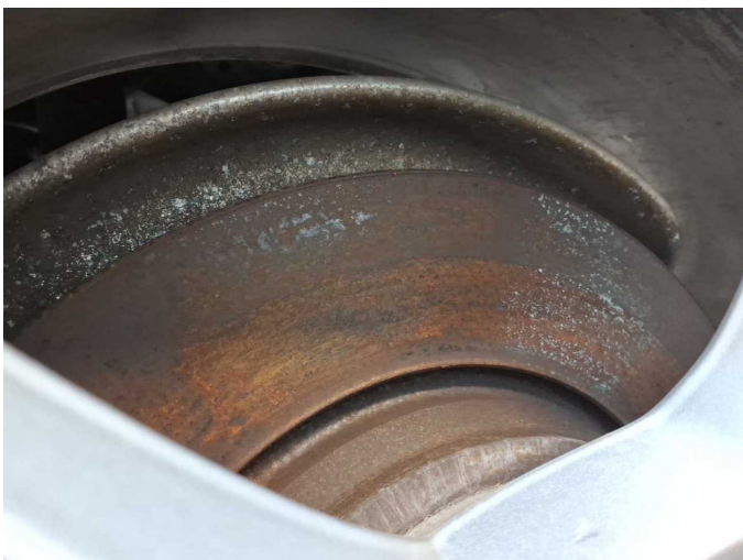
Damage 5: Braking system: Brake discs - front - Corrosion - Replace
