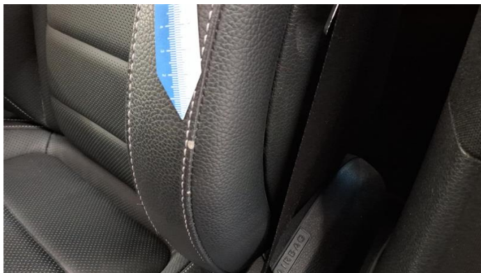
Damage 3: Seat - front: Backrest cover - left side - Scratch(es) - Smart repair
