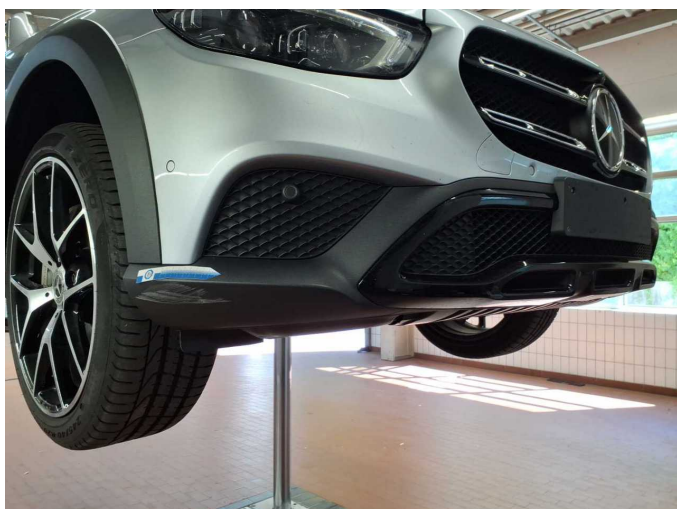
Damage 4: Front bumper: Spoiler - Scratched - Replace
