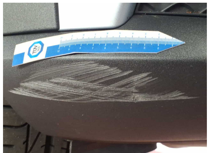
Damage 4: Front bumper: Spoiler - Scratched - Replace
