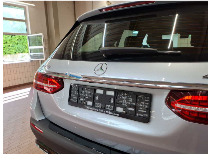
Damage 2: Boot lid / rear door: Protection strip - Scratch(es) - Replace
