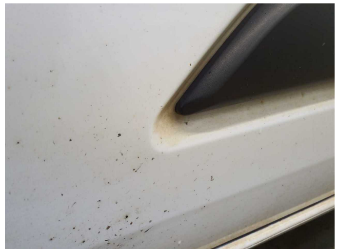
Damage 5: Body: Body (Flugrost) - Soiled - Clean
