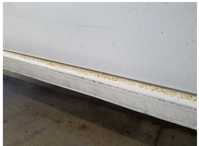
Damage 5: Body: Body (Flugrost) - Soiled - Clean
