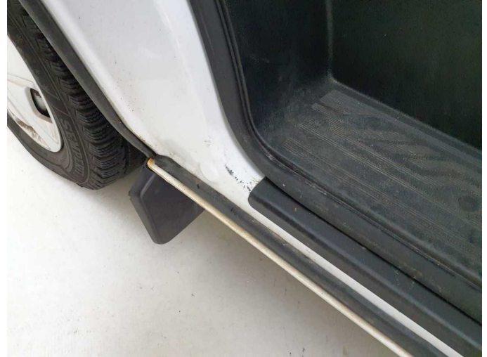
Damage 6: Sill - left side: Sill - Paint defect - Paint
