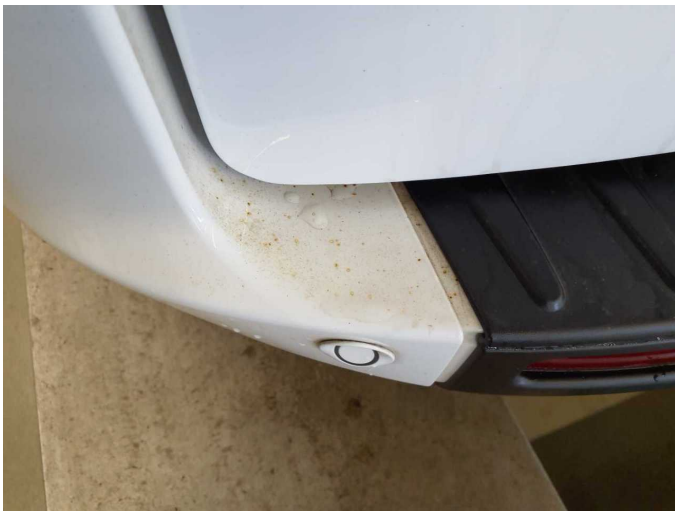
Damage 5: Body: Body (Flugrost) - Soiled - Clean
