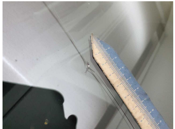
Damage 9: Vehicle glazing: Windscreen with lane departure assistant - Broken / torn - Replace
