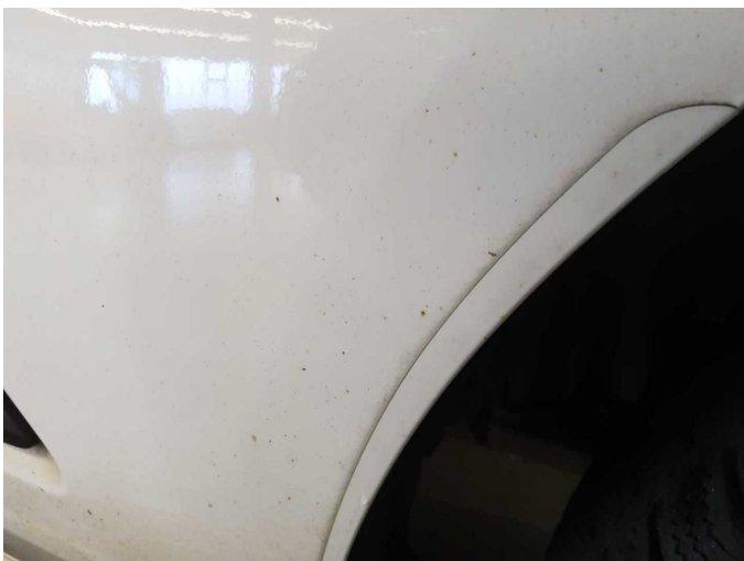
Damage 5: Body: Body (Flugrost) - Soiled - Clean
