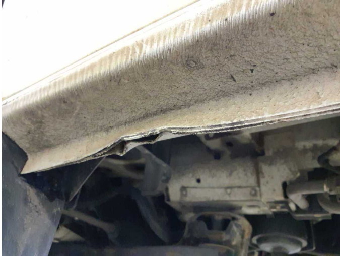
Damage 8: Sill - left side: Sill - Deformed - Repair and paint
