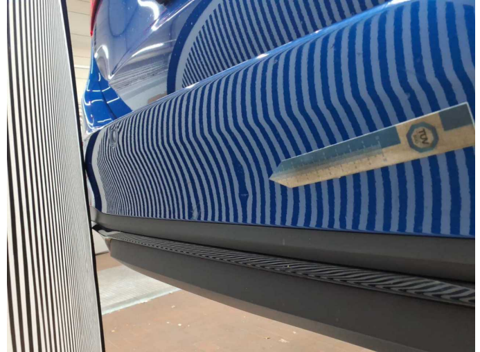
Damage 3: Rear bumper: Rear bumper - dent(s) - Loss in value
