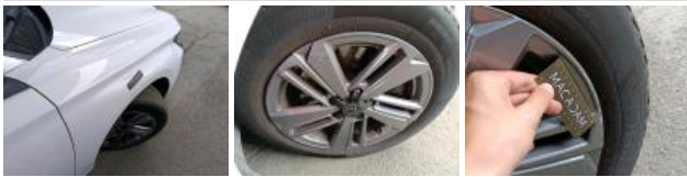
Tyre FR, Out of tolerance, Replace
