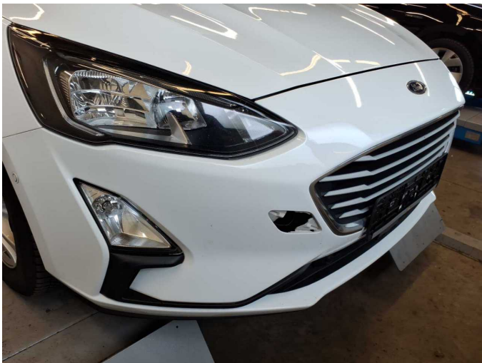
Missing part 1: Equipment: Towing eye - Missing - Replace
