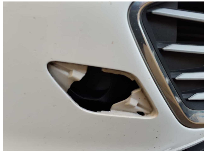
Missing part 1: Equipment: Towing eye - Missing - Replace
