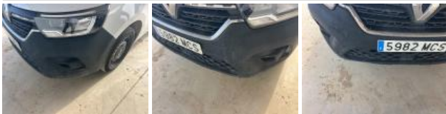
Bumper F, Dent(s) and scratch(es), Repair and paint (complete)
