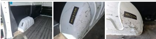
Wheel aperture RR, Dent(s) and scratch(es), Spot repair
