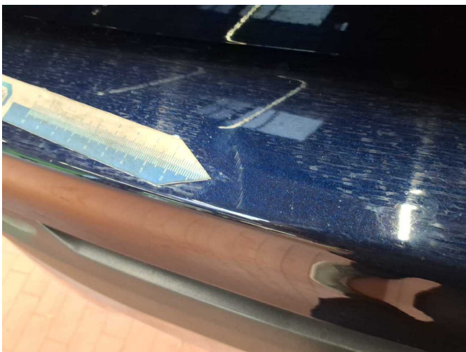
Damage 2: Rear bumper: Rear bumper - Scratch(es) - Smart repair
