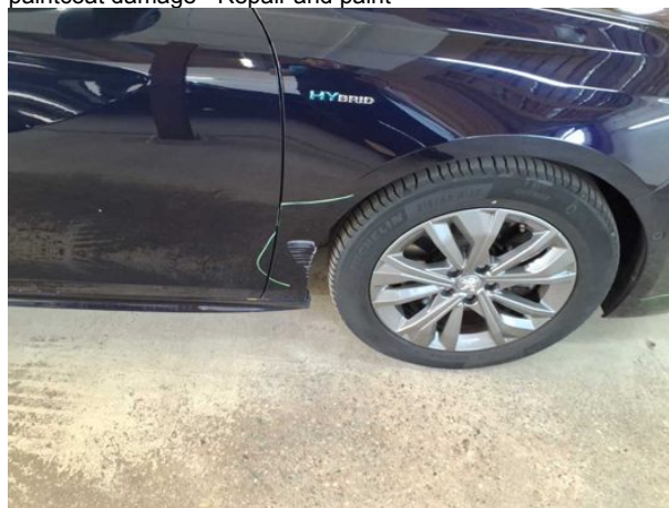
Damage #12: Mudguard - right side: Mudguard - right side - Deformed - Replace
