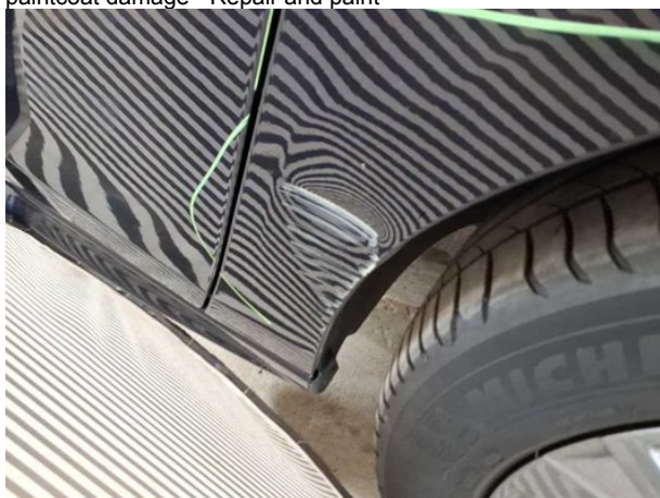
Damage #12: Mudguard - right side: Mudguard - right side - Deformed - Replace
