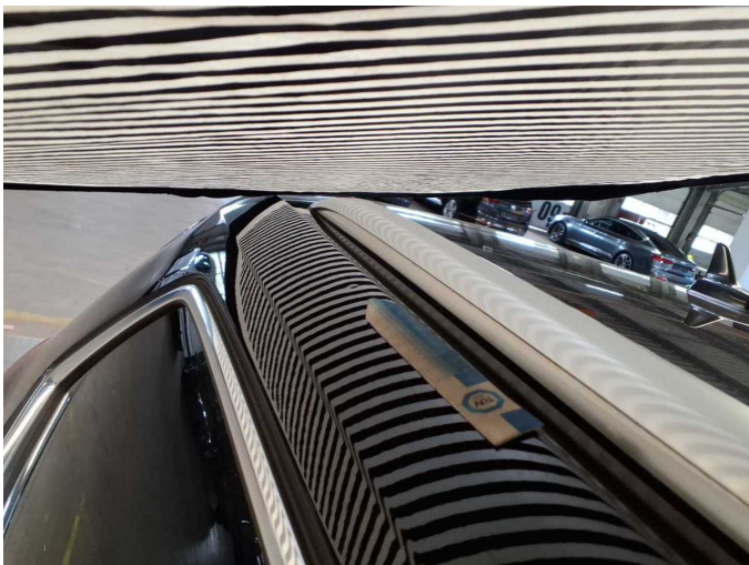
Damage 2: Roof: Roof rail - right side - dent(s) - Smooth repair work
