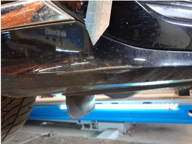
Damage 3: Front bumper: Spoiler - Scratch(es) - Smart repair
