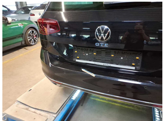
Damage 5: Rear bumper: Rear bumper - Scratch(es) - Smart repair
