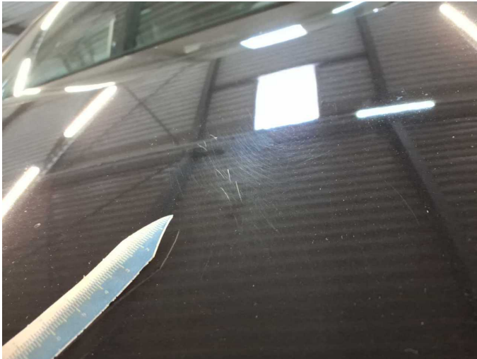
Damage 6: Bonnet: Bonnet - Scratch(es) - Paint
