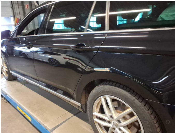
Wear and tear 3: Side panel - rear left side: Side panel - dent(s) - No deduction
