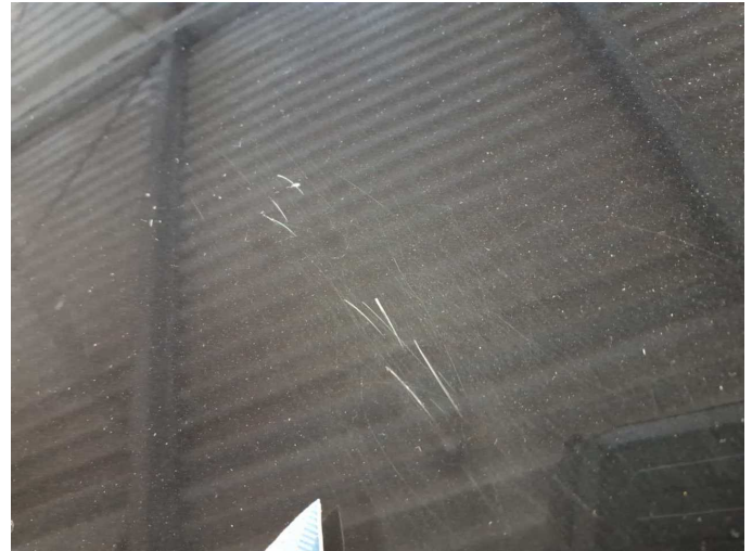
Damage 6: Bonnet: Bonnet - Scratch(es) - Paint
