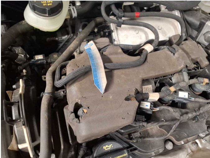
Damage 3: Misc.: Misc. (Isolierung Motor) - Damage caused by marten / rodent - Replace
