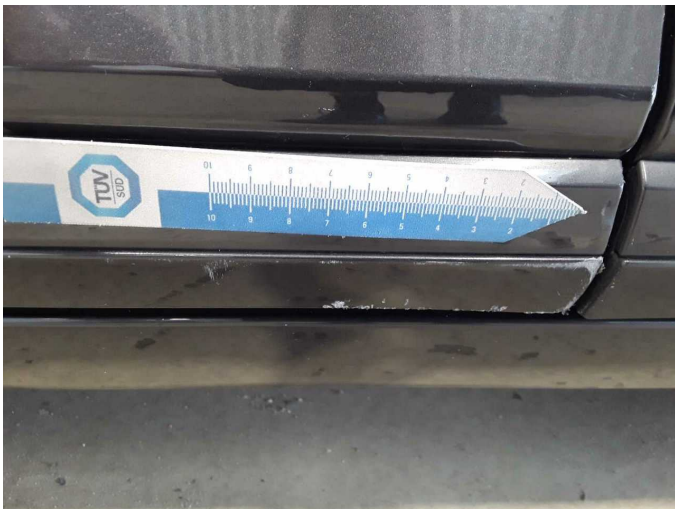
Damage 7: Door - front left side: Brightware - lower - Scratch(es) - Paint
