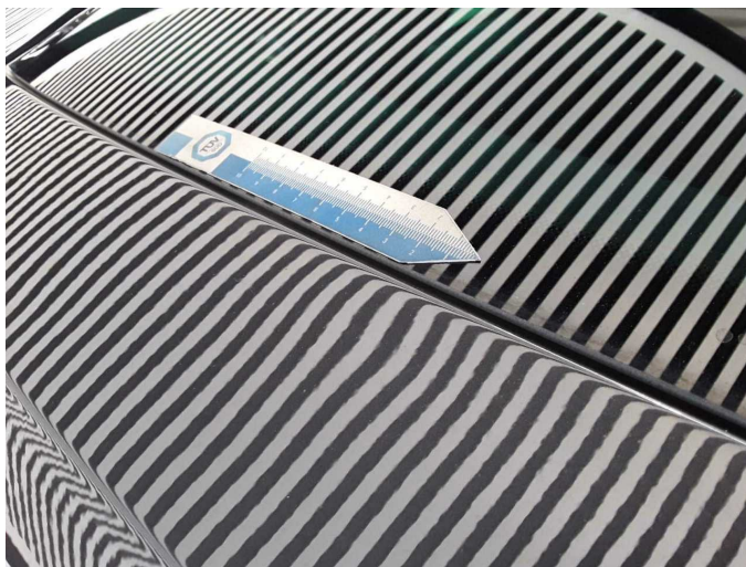
Wear and tear 4: Boot lid / rear door: Boot lid - dent(s) - Smooth repair work
