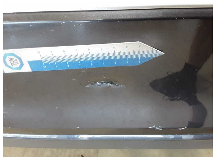
Damage 16: Rear bumper: Rear bumper - Broken / torn - repair according to calculation
