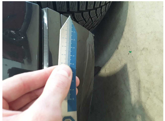
Damage 15: Front bumper: Front bumper - Scratch(es) - Paint
