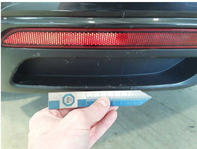
Damage 11: Rear bumper: Spoiler - Scratched - Replace
