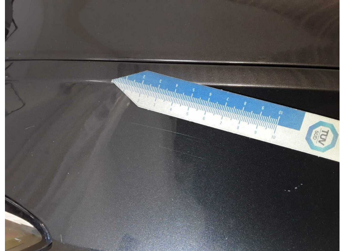
Damage 13: Mudguard - left side: Mudguard - left side - Scratch(es) - Paint
