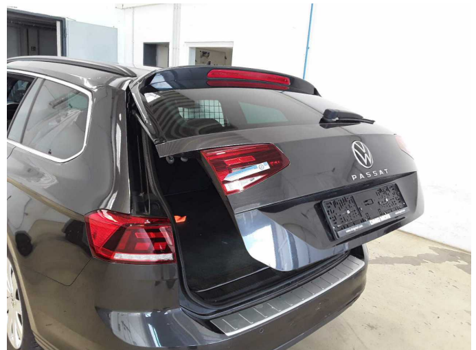
Damage 8: Tail light: Tail lamp - left side (Innen) - Broken / torn - Replace
