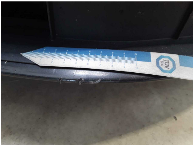
Damage 15: Front bumper: Front bumper - Scratch(es) - Paint
