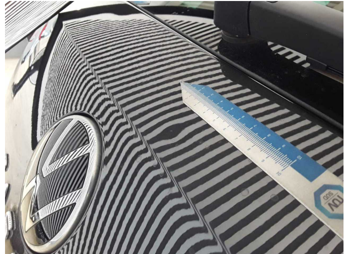
Wear and tear 4: Boot lid / rear door: Boot lid - dent(s) - Smooth repair work
