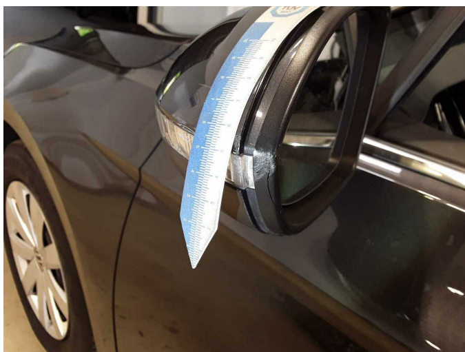
Damage 2: Wing mirror - left side: Mirror housing (Blende) - Broken / torn - Replace
