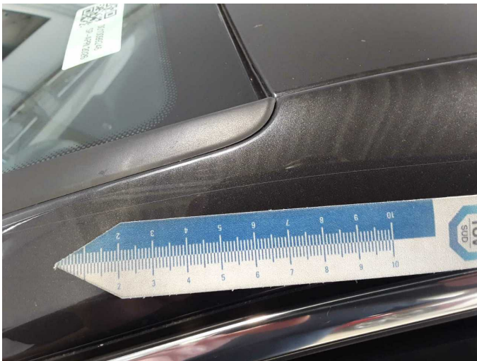
Damage 10: Roof: Roof rail - left side - Scratch(es) - Paint
