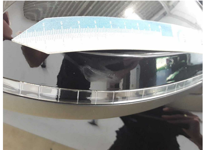
Damage 2: Wing mirror - right side: Cap - Abrasion - Smart repair
