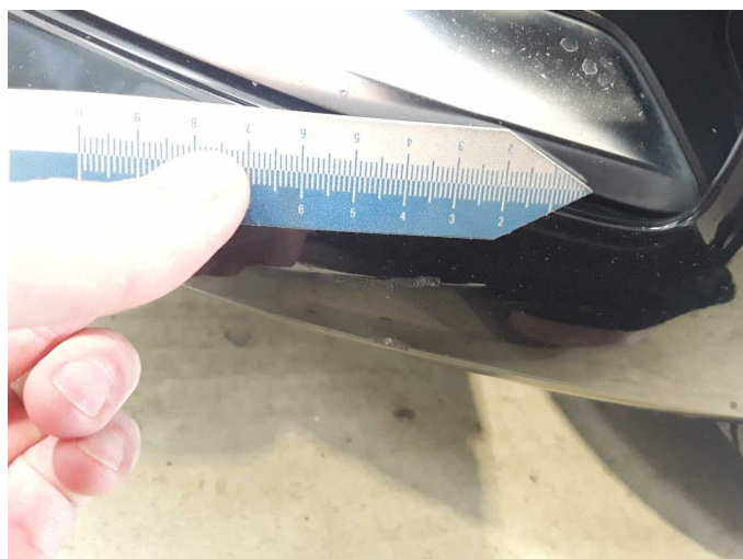
Damage 5: Front bumper: Front bumper - Scratch(es) - Paint
