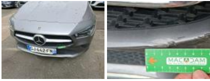
Bumper F, Deformed / Strained, Repair and paint (complete)
