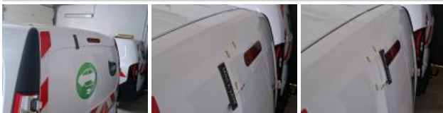
Boot door panel RR, Dent(s) and scratch(es), Acceptable
