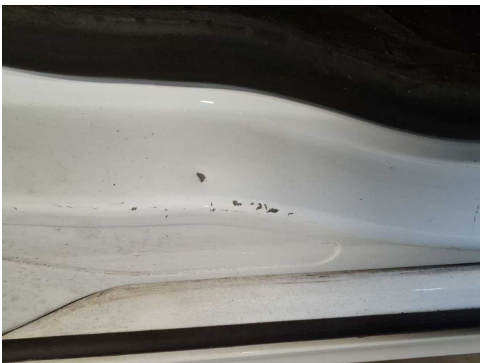
Damage 12: Side panel - rear right side: Sill - Dent / paintcoat damage - Smart repair
