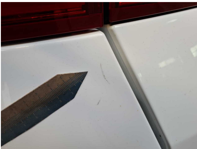
Damage 20: Rear bumper: Rear bumper - Scratched - Paint
