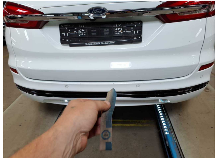
Damage 20: Rear bumper: Rear bumper - Scratched - Paint
