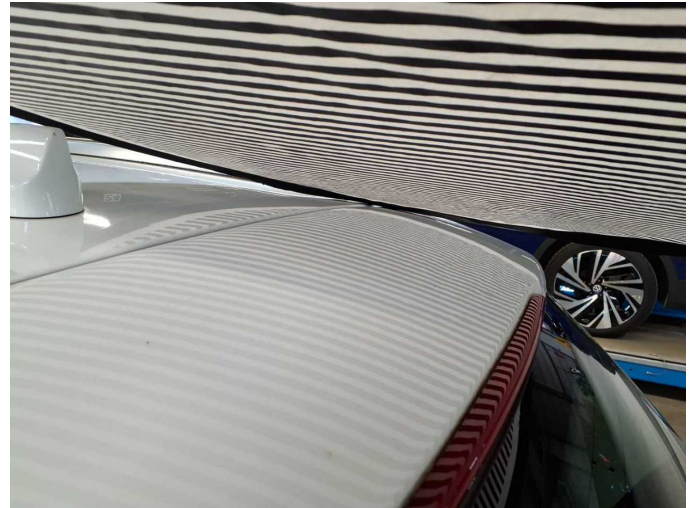
Damage 21: Body: Body (+ Motorhaube Lackschaden) - Damage by hail - Smooth repair work
