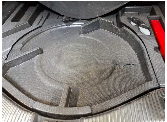
Damage 8: Interior: Cargo area floor (Abdeckung) - Broken / torn - Replace
