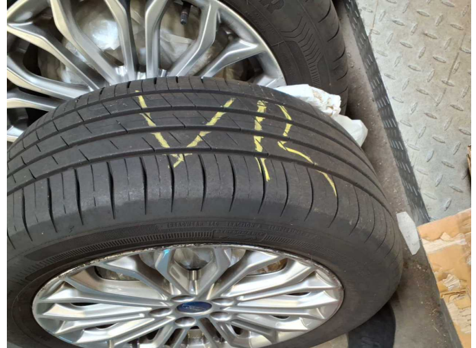
Damage 7: 2nd wheel set: 1 tyre (Flanke) - Damaged - Replace
