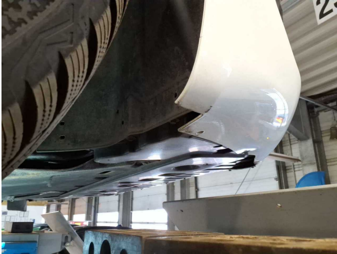
Damage 3: Mudguard - right side: Mud flap (Schmutzabweiser) - Missing - Replace
