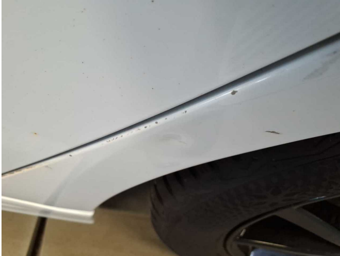
Damage 18: Side panel - rear left side: Side panel - Dent / paintcoat damage - Repair and paint
