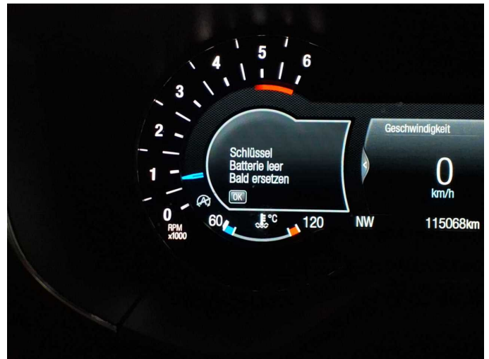
Damage 1: Equipment: Vehicle key (Batterie) - Empty - Replace
