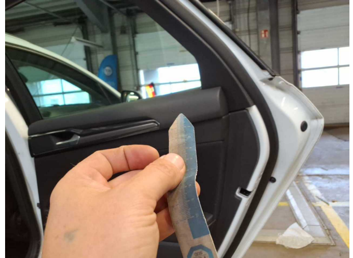
Damage 11: Trim / covers: Door trim - rear right side - Damaged - Smart repair
