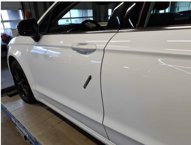
Damage 17: Door - front left side: Door - Dent / paintcoat damage - Repair and paint
