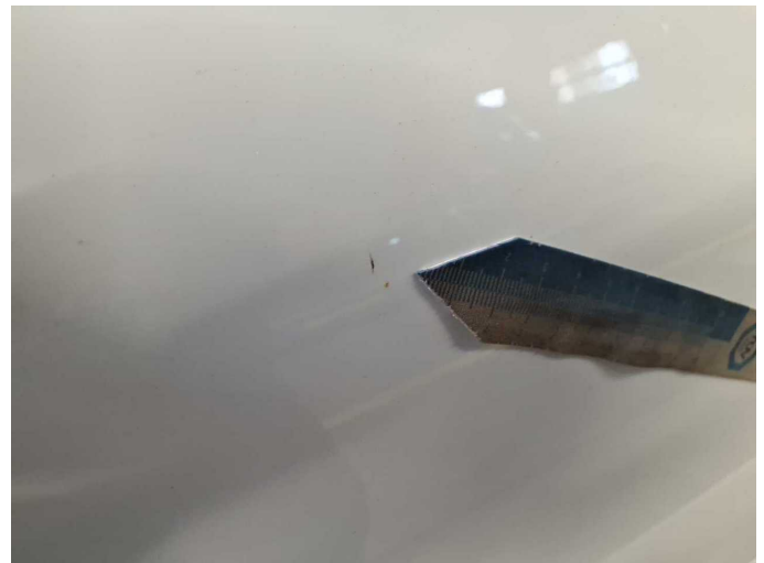
Damage 16: Door - rear right side: Door - Scratch(es) - Paint
