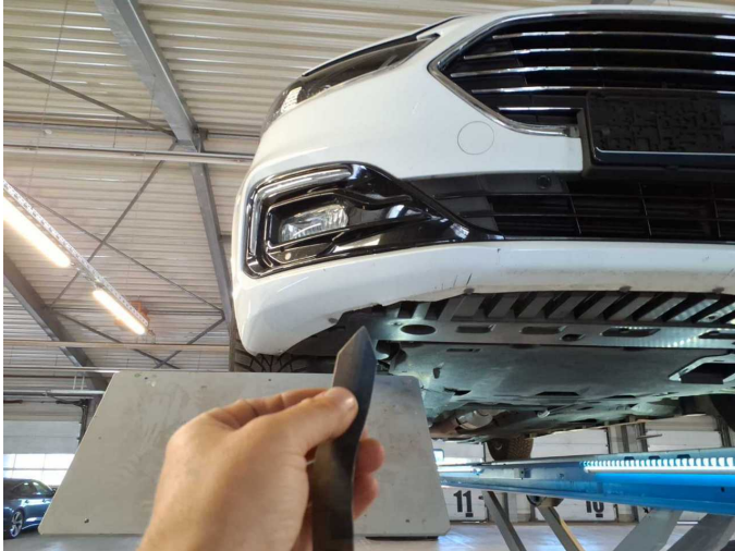
Damage 19: Front bumper: Front bumper (Verformt) - Scratched - Repair and paint
