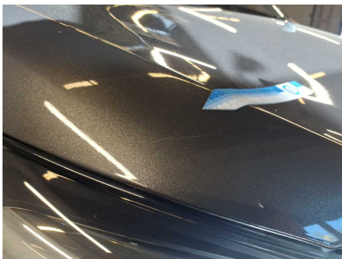
Damage 5: Bonnet: Bonnet - Scratched - Paint
