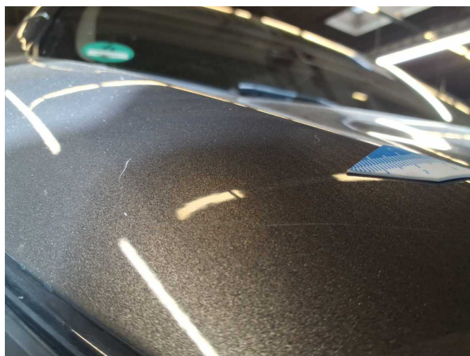
Damage 5: Bonnet: Bonnet - Scratched - Paint
