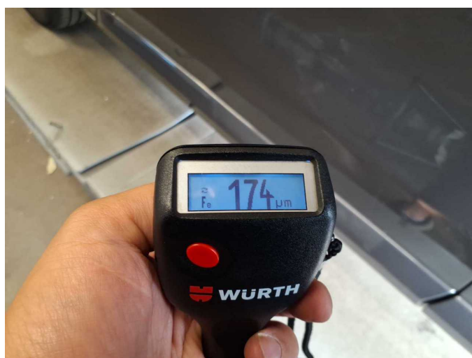
Repainting 1: Roof, Door - rear right side, Door - front right side
