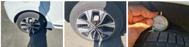
Tyre FR, Out of tolerance, Replace
