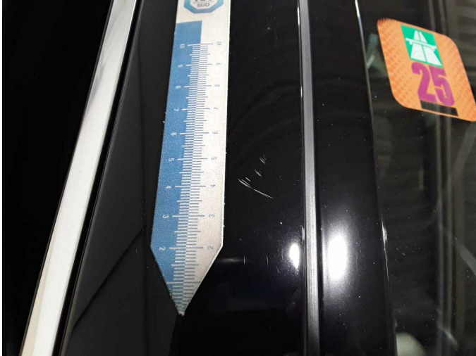
Damage 3: Body: A-pillar - right side - Scratch(es) - Smart repair
