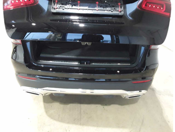
Damage 4: Rear bumper: Rear bumper (LadeKante) - Scratch(es) - Smart repair
