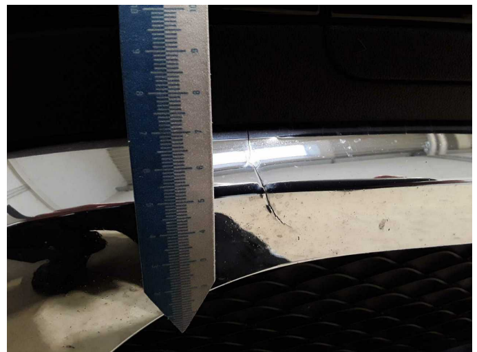
Damage 5: Front bumper: Cover bumper - front - Broken / torn - Replace
