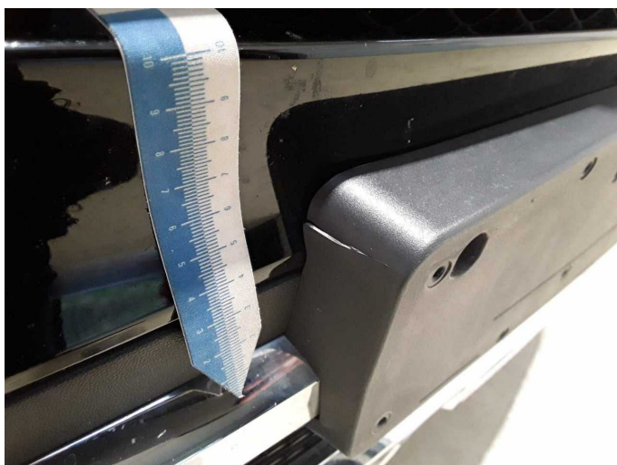
Damage 1: Front bumper: Licence plate holder - Broken / torn - Replace
