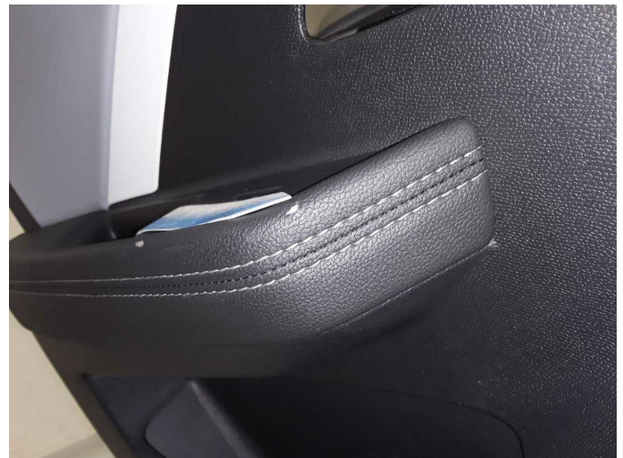
Damage 6: Trim / covers: Door trim - rear left side - Scratch(es) - Smart repair
