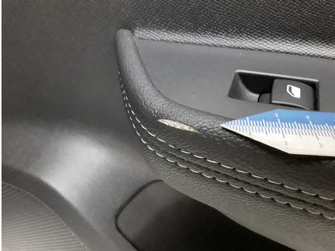
Damage 5: Trim / covers: Door trim - rear right side - Scratch(es) - Smart repair
