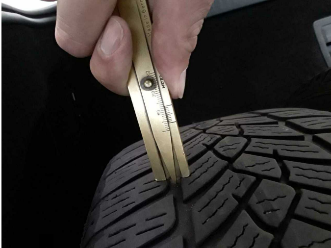
Damage 8: 2nd wheel set: 3 tyres - Does not meet the leasing specifications - Replace
