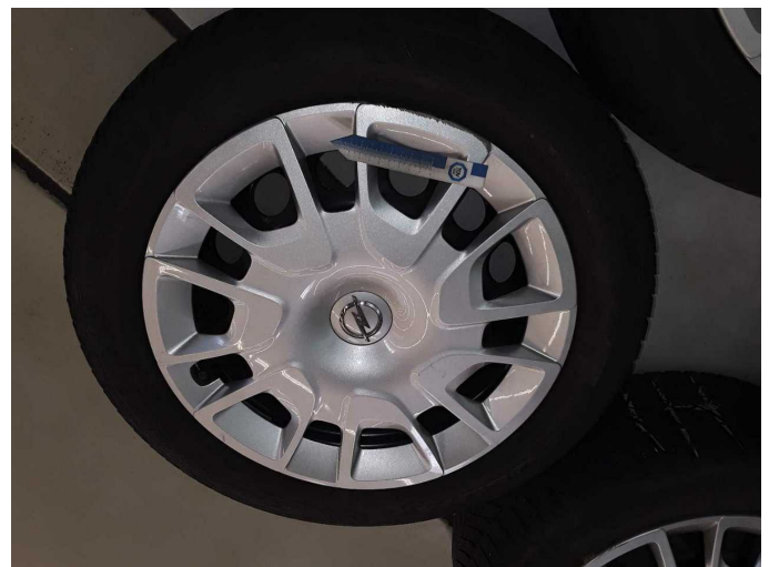
Damage 2: 2nd wheel set: 1 wheel cover - Broken / torn - Replace
