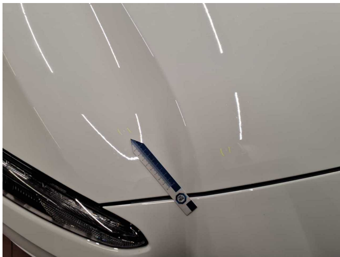
Damage 6: Bonnet: Bonnet (Lackeinschlüsse) - Unprofessionally repaired - Paint
