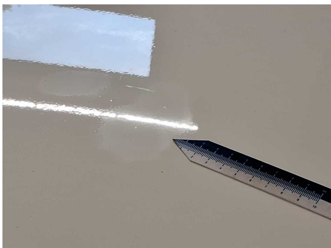
Damage 6: Bonnet: Bonnet (Lackeinschlüsse) - Unprofessionally repaired - Paint
