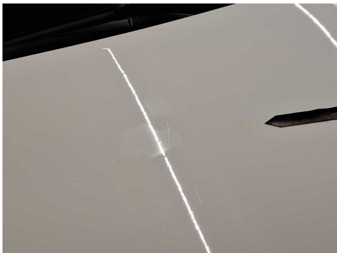
Damage 6: Bonnet: Bonnet (Lackeinschlüsse) - Unprofessionally repaired - Paint
