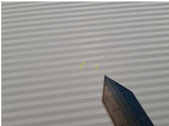
Damage 6: Bonnet: Bonnet (Lackeinschlüsse) - Unprofessionally repaired - Paint
