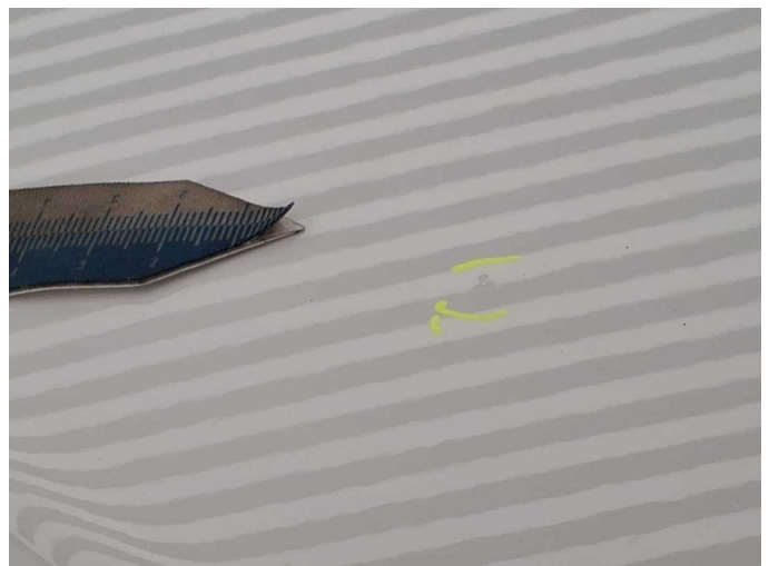
Damage 6: Bonnet: Bonnet (Lackeinschlüsse) - Unprofessionally repaired - Paint
