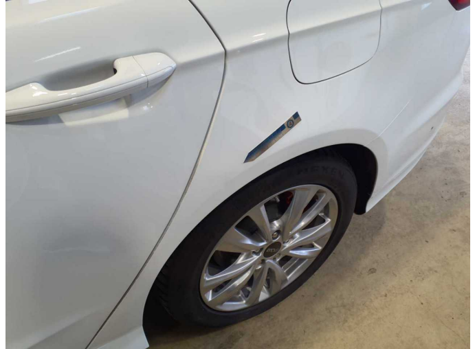
Damage 8: Side panel - rear left side: Side panel - dent(s) - Repair and paint
