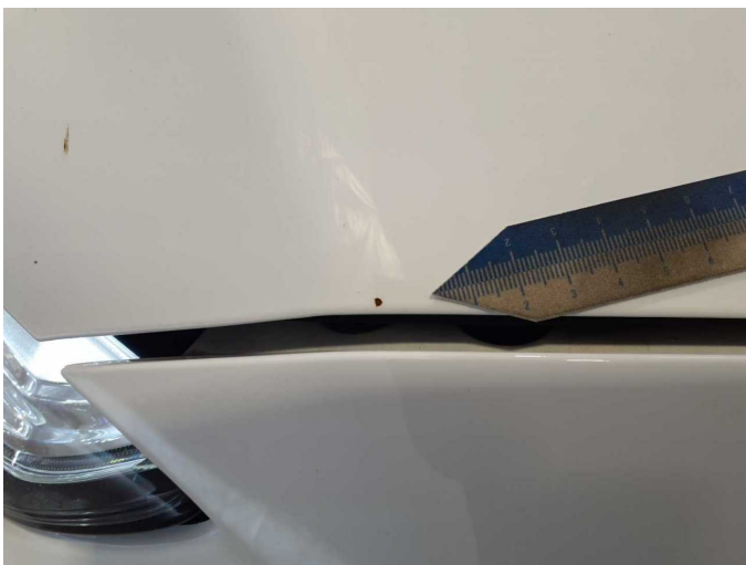
Damage 9: Bonnet: Bonnet - Corrosion - Repair and paint
