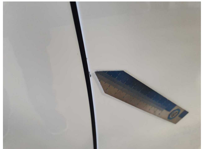
Damage 3: Door - front right side: Door edge - Scratched - Smart repair
