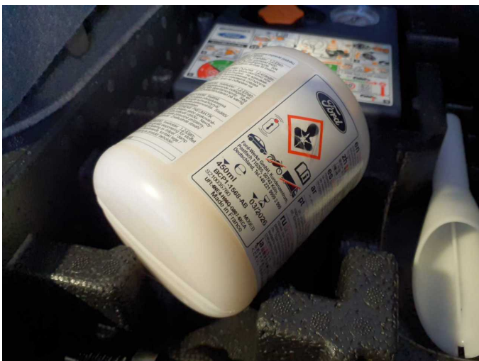
Damage 4: Equipment: Tirefit filler - Expired - Replace
