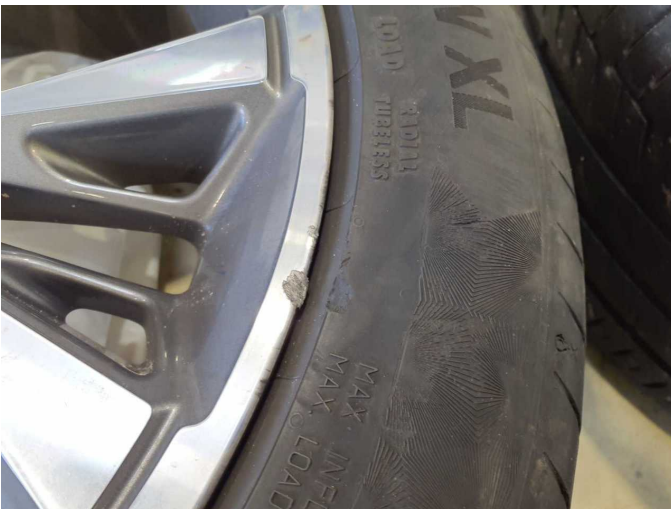
Damage 6: 2nd wheel set: 1 tyre - Damaged - Replace
