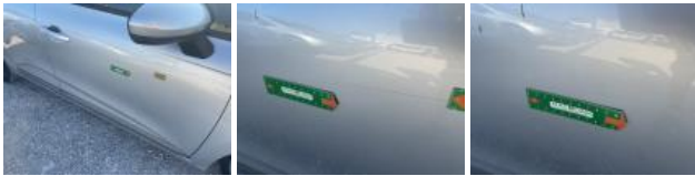
Door RR, Dent(s), Repair and paint (complete)
