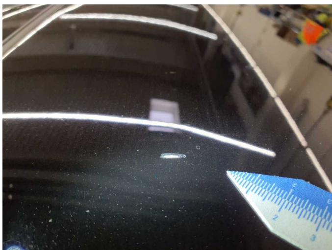
Damage 1: Roof: Roof - Dent / paintcoat damage - Smart repair
