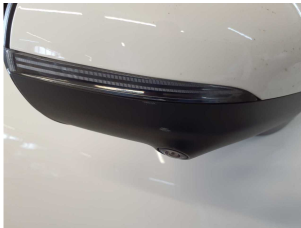
Damage #1: Wing mirror - right side: Mirror housing - Scratch... - Loss in value
