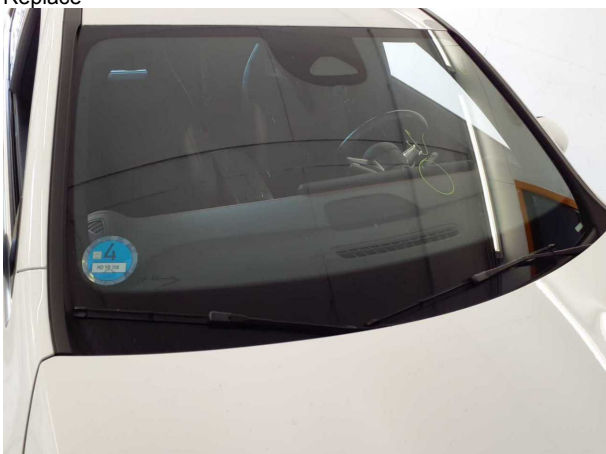
Damage #7: Vehicle glazing: Windscreen - Stone chips - Replace
