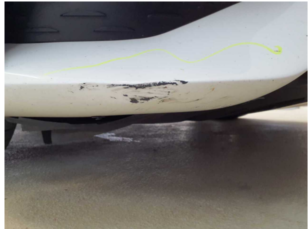
Damage #8: Front bumper: Front bumper - Dent / paintcoat damage - Repair and paint
