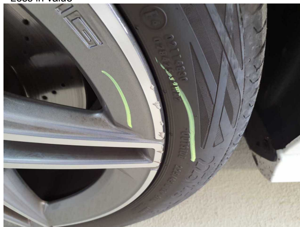
Damage #2: Wheel / tyres: Alloy rim - front left side - Scratched - Loss in value
