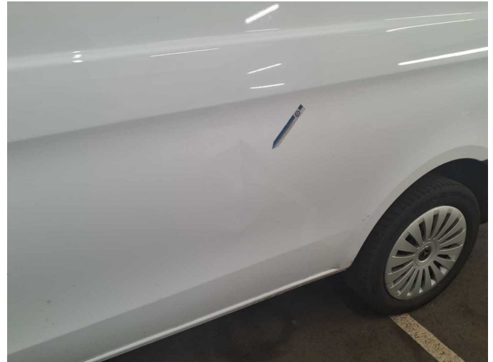
Damage 1: Side panel - rear left side: Side panel - Deformed - Repair and paint
