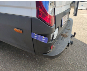
Bumper Rear / Lower Cover Not Painted / Replace-scratch
