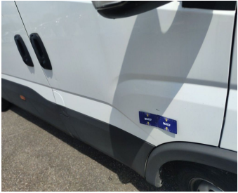
Door Front Right // Repair & Painting-scratch + dent
