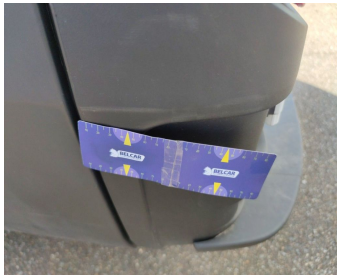
Bumper Rear / Lower Cover Not Painted / Replace-scratch
