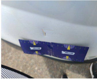
Bumper Front // Repair & Painting-scratch + dent
